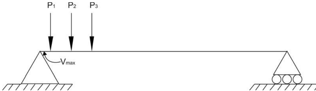
Figure 8.23: Absolute maximum shear – simply supported beam
