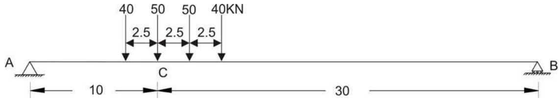
Figure 8.18: Beam loaded with a series of loads – Second load at section C
