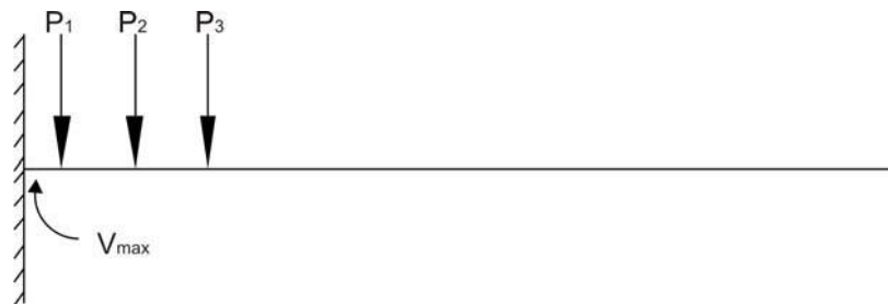
Figure 8.22: Absolute maximum shear case – cantilever beam
