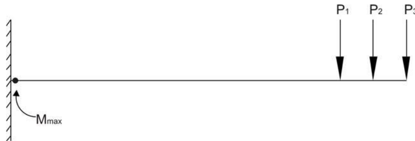
Figure 8.24: Absolute maximum moment – cantilever beam
